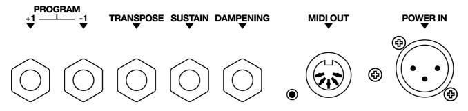
Plug the power supply unit into a wall socket and the XLR connector into the instrument (power in). There is no on/off switch. If you have internal sounds just plug in your headphones or line out to PA and start playing. Or, using the supplied MIDI lead, connect the MIDI Out socket on the Xylosynth to the MIDI In socket on your sound source. Then run up and down the keyboard to make sure all the keys are activated.
